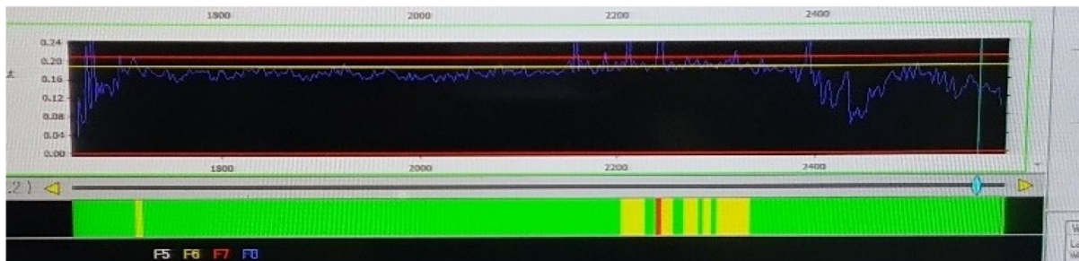
Fig.6. The curve is very close the upper limit (dark line) , but this welding seam quality was judged “okay” by the judgement system.
