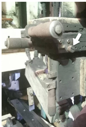
Fig.1. The lock screw of the filler wire unit.
